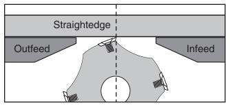
**Figure 57.** Infeed table adjusted even with outfeed table.
